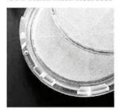
The new gold plated, copper mesh electrodes have a very fine weave, yet allow extraordinarily free air passage. This unique material also resists vibration while its shape limits reflections back to the 1.5 micron polyester diaphragm. These characteristics achieve transparent reproduction of even the most delicate notes.
